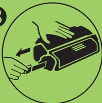
3. Pull out the sealing tape slowly with horizontal force to avoid breaking of sealing tape.
