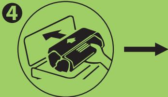
4. Install the laser toner cartridge into the printer in the direction as showed by the arrow on the cartridge.
