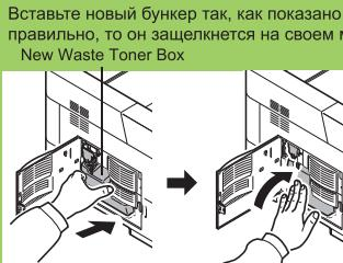
**7** Make sure that the waste toner box is correctly inserted and close the left cover.
